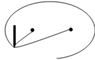
Figure 7: A simpler way to construct an ellipse
